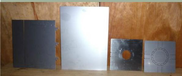
*A complete LuciaStove is ready for assembly. The stove ships flat-packed to Rwanda where the stainless steel sheets are rolled, bent, and welded into a finished LuciaStove.*
