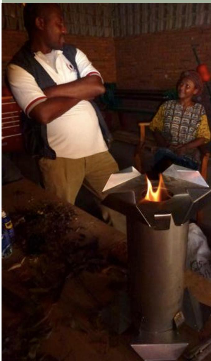
*LuciaStoves pyrolyze fuel pellets made from Rwandan biomass and burn as a clean & hot gas flame ([video here](#)). Above, the first LuciaStove to burn Inyenyeri’s Rwandan fuel pellets.*
